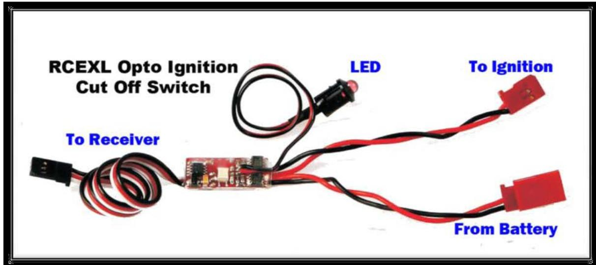
It is another safety device that hopefully will never be needed by its user. But in that one in a million chance that you need to stop an engine quickly - outside of crashing the plane - having this switch in place will make it all worthwhile.
