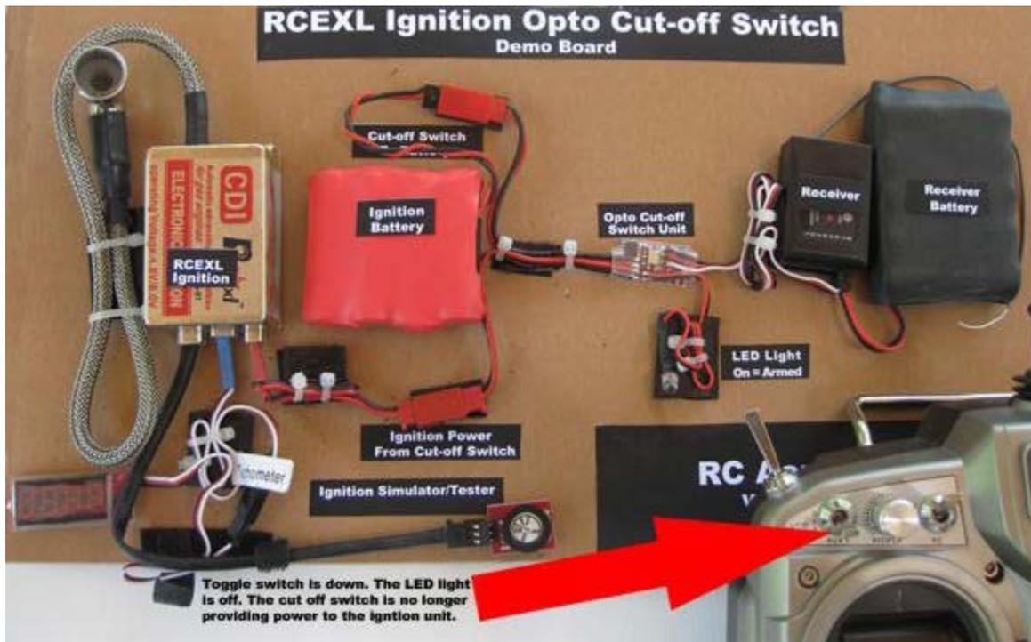
In this picture, the toggle switch on the transmitter is in the DOWN position,(red arrow) which in this case means the power is OFF. The LED light is OFF. The ignition module
