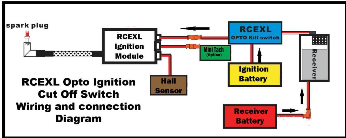
On the newer RCEXL ignition modules, you will see 4 cables running from the unit. The older units have only 3. Attaching the ignition cutoff switch to the ignition module needs only connection - the battery (Power in) connector. This cable is the conduit that supplies the necessary power to the ignition unit.
