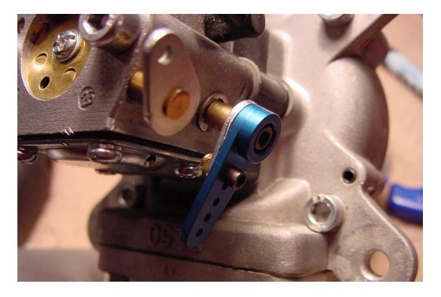
If you are like me, you dread the thought of receiving a new gas engine and immediately finding out the Walbro carb has a throttle arm to small to use. Coming up with a workable solution has always been a pain.
