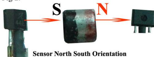
Insert fully the sensor into the sensor housing. Use the supplied wedge to hold the sensor in its housing. (fig. 3) **Warning!!** The wedge provides a one way fit; make sure you have the proper sensor orientation before inserting the wedge as it will be very difficult to remove!
