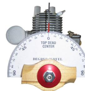
Turn the crankshaft clockwise (opposite to the engine rotation) until the wheel reads 28 degrees.
