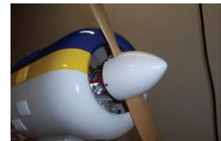
4. Place the spinner on the backplate, making sure to line up the screw holes with the mounting risers on the backplate. Now place the template onto the spinner between the mounting screws, making sure that the bottom edge of the template sits along the bottom edge of the spinner.
