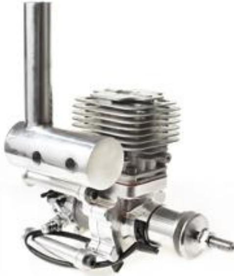
Two items important to remember with any engine. The needle settings required to get most any engine started is between 1-1/2 to 2 turns open on both needles. The second is never try to tune or adjust a cold engine. They must be warm for a needle or idle setting to be effective. Otherwise the effects of changed settings alter as an engine warms up.
