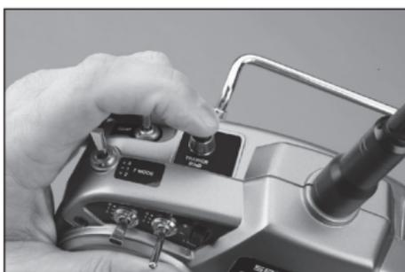
4. Follow the procedures of your specific transmitter to enter Bind Mode, the system will connect within a few seconds. Once connected, the LED on the receiver will go solid indicating the system is connected.
