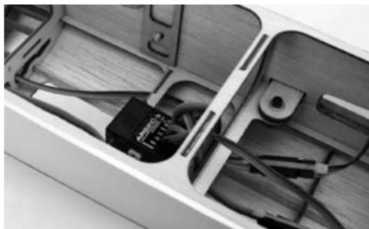
In helicopters, there is generally enough room on the servo tray to achieve the necessary separation. If necessary a mount can be fashioned using clear plastic to mount the external receiver.
