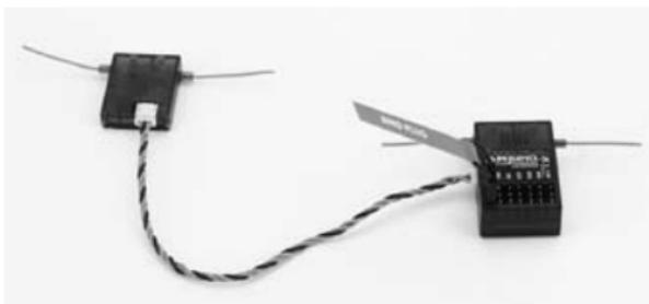
**Note:** To bind an aircraft with an electronic speed controller that powers the receiver through the throttle channel (ESC/BEC), insert the bind plug into the BIND/DATA port in the receiver and the throttle lead into the throttle (THRO) port. Proceed to Step #2.
